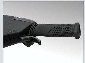
iBR™ (Intelligent Brake & Reverse) brake lever
