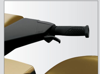
iBR™ (Intelligent Brake & Reverse) brake lever
