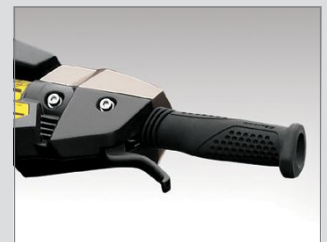
iBR™ (Intelligent Brake & Reverse) lever
